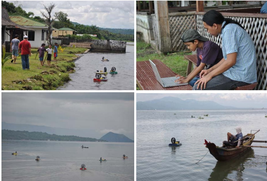
Fig. 7. Our six week deployment in the Philippines demonstrated an ability to deploy five airboats simultaneously in remote locations with a control interface simple enough to be used by a child.
